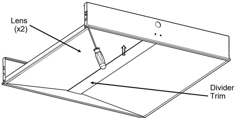
1. Begin at the side of the housing flange where it meets the end plate. Use flat screwdriver and gently pry back the lens and use fingers to remove.
