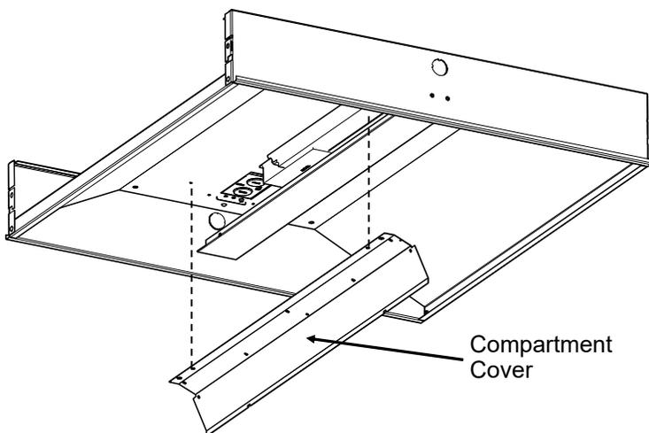
1. Select one of the two compartment covers. Remove 2 screws to gain access to driver compartment.
