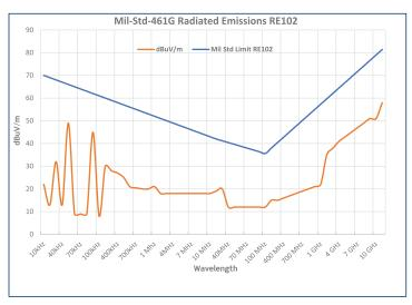
Conducted measurements are taken from the fixture power input leads in a laboratory. Radiated emissions are measured in an anechoic chamber designed to absorb indirect signals from the environment. The limits are shown in the red lines. Performance is shown on the yellow line. For more information on Mil-Std-461G see the Certolux Technical Brochure. Click here
