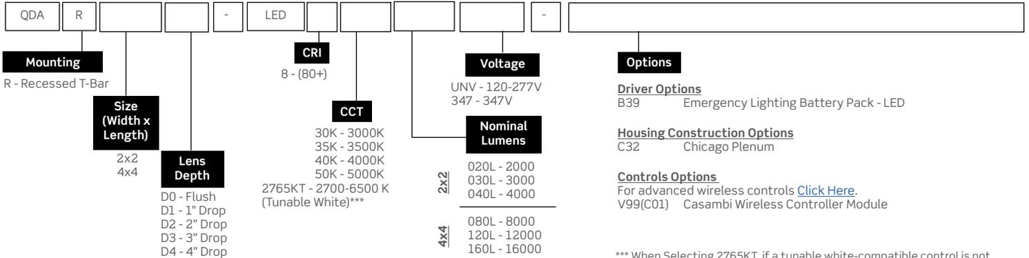
\*\*\* When Selecting 2765KT, if a tunable white-compatible control is not selected the luminaire will come standards with two sets of 0-10V wires for dimming and color tuning (see tunable white diagram for details). For compatible control options please consult factory.
